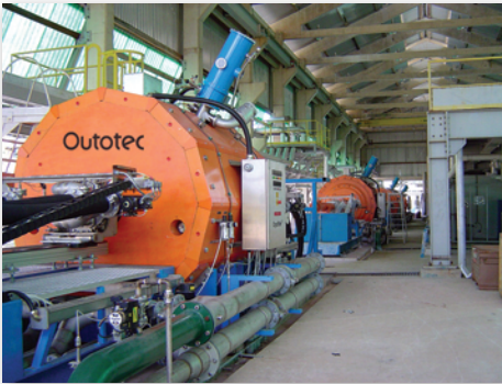
Industrial LTS Magnetic Separator Image courtesy of Outotec (USA) Inc.
