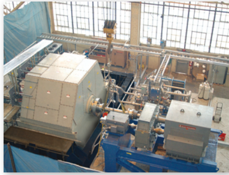
36.5 MW HTS Ship Drive Motor Image courtesy of American Superconductor
