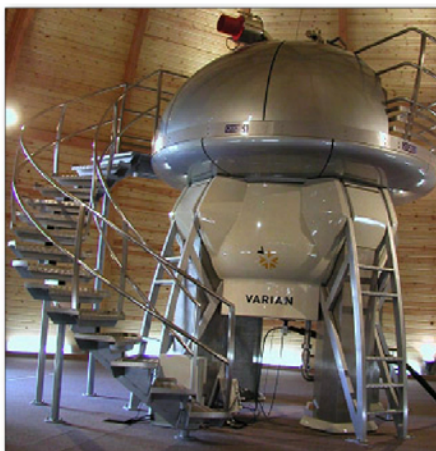
A 900 MHz NMR spectrometer
